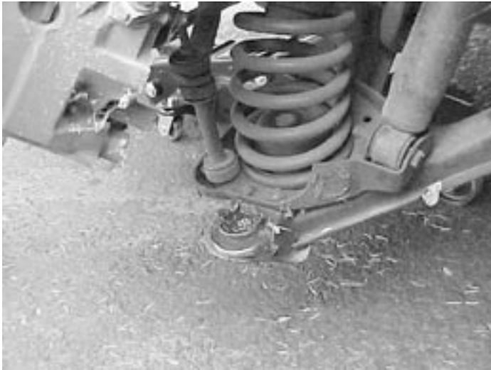
The Lower Ball Joint Has a Clean Break
