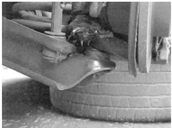
The A-Frame is Not damaged.
