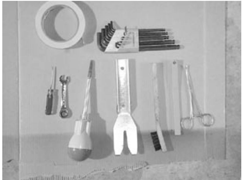
Fig 1: Tools for replacing dew-wipes (outer seal strip).
